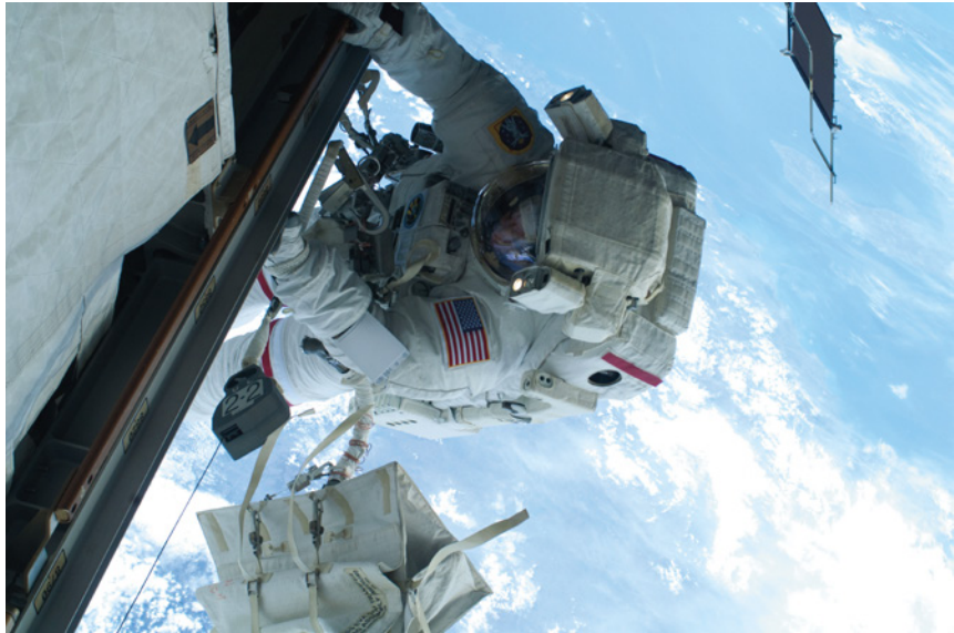
Figure 1-1: NASA astronaut Rick Mastracchio on a 26-minute spacewalk in 2010, as photographed by astronaut Clayton Anderson. The spacewalk outside the International Space Station was one of a series to replace coolant tanks.
